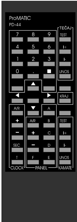
Digits, arrows, KRAJ (END) and keys in frame “TEČAJ” and “CLOCK” are used for entry data to exchange rate board.
